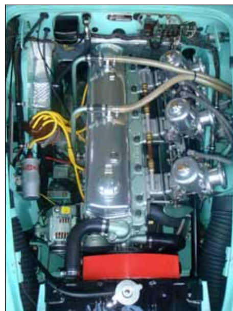
The Business End of Things ... The big 6-cylinder sporting a period Ruddspeed manifold and race tuned triple 2" SU HD8 carburetors. Doug's engine is built for speed without sacrificing reliability.
